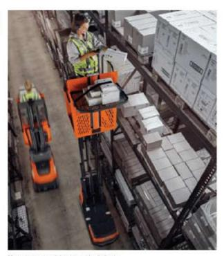
\* Certain options or country standards may increase weight and/or dimensions. \*\* Maximum driving speed allowed up to 0,5m (platform floor height) \*\*\* At maximally elevated platform speed up to 1.6 km/h
