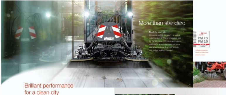
Sweeping is one of the main tasks in the field of Municipal Technology. The Citymaster 650 carries out all aweeping tasks rapidly, reliably and efficiently: thanks to its hydraulsally driven 2-broom aweeping unit, quick-change suction duct and Intelli-Flap\* coarse dirt flap. The machine's patented circulation water system provides maximum dust control – and ensures clean exhaust air and lowest possible dust and fine particulate emissions.
