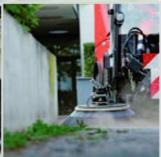
Gets in almost every corner: The steering system with articulated joint ensures excellent manoeuvrabilityven when sweeping in reverse gear.
