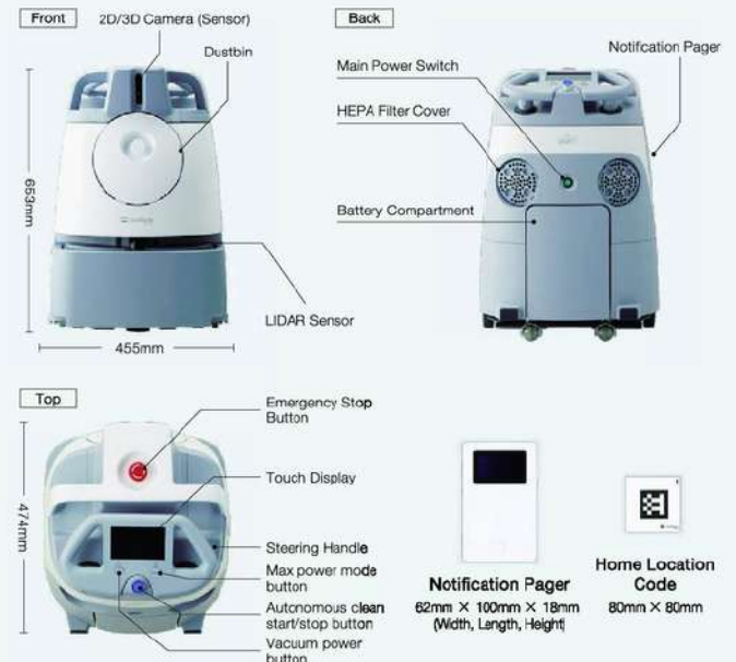
HEPA Filter Captures 99.97% of PM2.5 particles, including pollen and house dust
