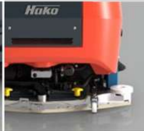
Optimal intake of dirt water via the squeegee.
